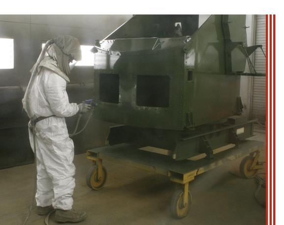
Using a high volume, low pressure paint gun, a depot painter sprays chemical agent resistant coating over an AN/TWQ-1 Avenger gunner's turret. Letterkenny's advanced paint mixing system reduces labor, cost, and waste. The materials used are at the lowest volatile organic compounds (VOC) that still meet the military specifications and are more environmentally friendly.
